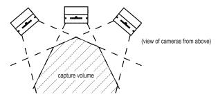
6. Run the Tracking Tools software and start a camera calibration. Slowly move the wand throughout the entire capture volume, in a circular pattern. Save the resulting calibration to a file for later use.
